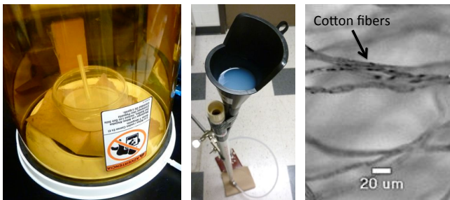
Figure 1. Degassing polymer to remove air bubbles before casting process (left). PVC and copper casting mold to make compliant polymer tubes (center). Microscope image of experimental AT fibers at 40x magnification (right).
