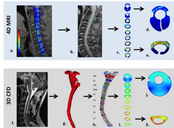
**Figure 2.** Study methodology diagram. 4D pc MRI measurement (a) and flow quantification (b,c,d & e). 3D CFD simulation: MRI measurement of geometry (f), 3D reconstruction of geometry (g), CFD simulation (h) and measurement plane comparison (i, j & k) [2].
